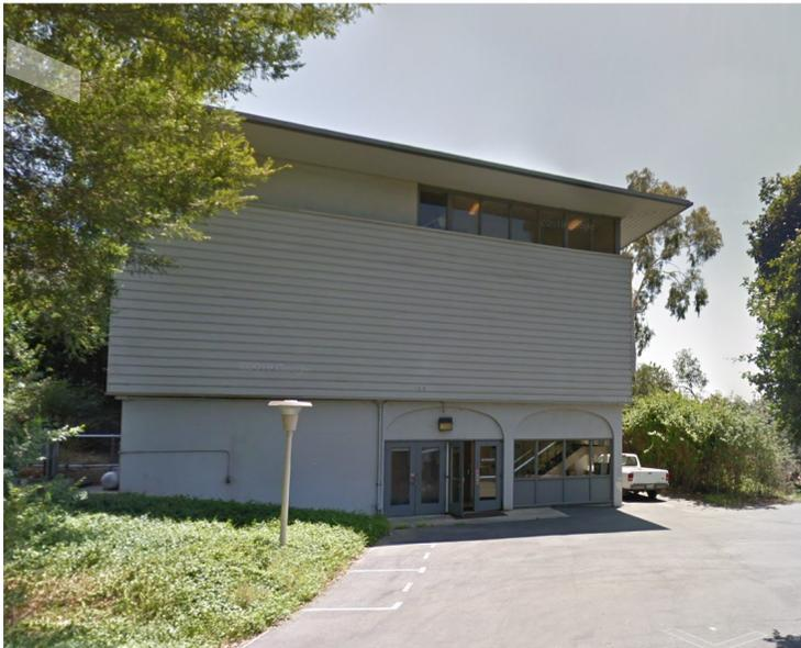
In response to the UC Seismic Safety Policy update of May 2017, UCR completed its first phase of seismic building assessments in early 2019. College Building North was assessed by an independent structural engineering consultant and rated as a “V” on a scale of “I” (best anticipated performance in a major seismic event) to “VII” (anticipated to be very unsafe in a major seismic event).
